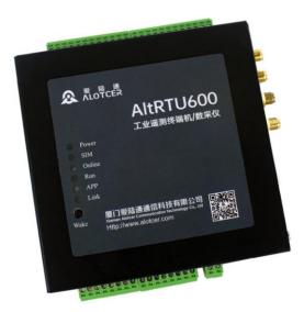
AltRTU600L is an industrial cellular RTU developed based on 5G/4G LTE connectivity. It adopts high-powered industrial 32 bits CPU and industrial wireless module, and embedded real time operating system to realize comprehensive functions such as data acquisition, storage, control, alarm, remote transmission and remote management.
